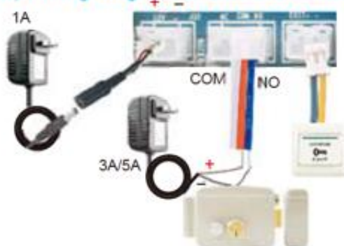
Power on wiring diagram
