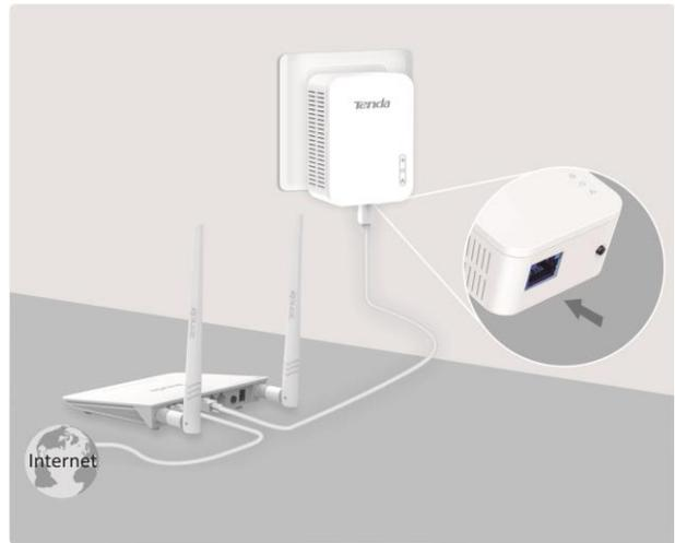
**Step 2** Plug PA6 into a wall receptacle near the router.
